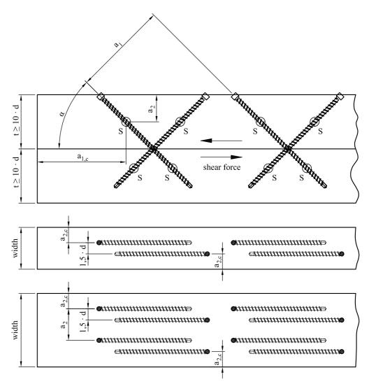
S = centroid of the part of the screw in the timber
