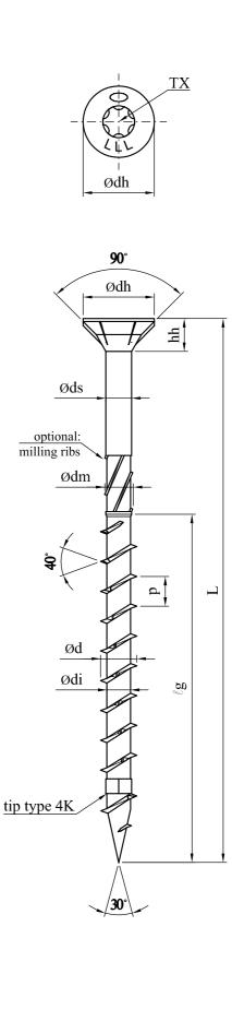
All dimensions in mm. \* max. L for d= 6,0/8,0/10,0 mm
