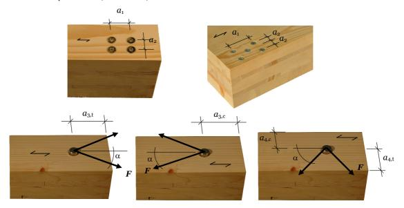
Figure 2: Definition of spacing, end and edge distances in the edge surface unless otherwise specified in the technical specification (ETA or hEN) for the cross laminated timber:
