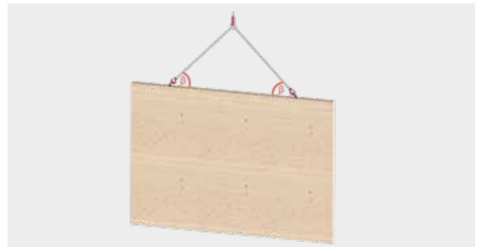
Vertical CLT wall or beam
