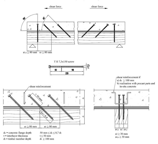
Table 1.1 – Minimum spacing, end and edge distances for T II 7,3x150 screws in mm
