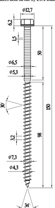
ANNEX 3 Drawing of the T II 7,3x150 Screw Tolerances held on file by ETA-Danmark A/S
