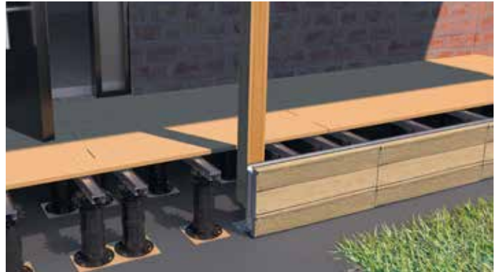
12 The terrace decking boards are laid parallel to the house façade. Laying is started with the first board next to the house façade. In our example, we have chosen a visible fastening and screwed the decking boards to the EVO aluminium system profiles with the Eurotec profile drilling screw . As tools, we recommend the drill-stop , the spacers and the tension clamp .
